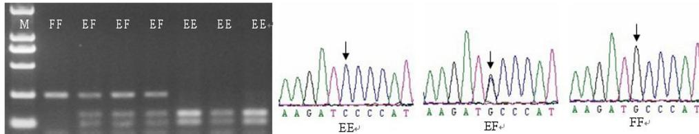
**Figure 3.** Agarose gel electrophoresis of *Mbo*I PCR-RFLP. The EE genotype shows 2 fragments (143 and 101 bp), the EF genotype shows 3 fragments (244, 143 and 101 bp) and the FF genotype shows 1 fragment (244 bp). Lane M = DNA marker, DL2000 (TaKaRa, Dalian, China).
