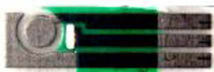
Figure 1. Appearance of disposable electrochemical printed (DEP) chips, round working electrode type EP-N (Biodevice Technology, Ishikawa, Japan).
