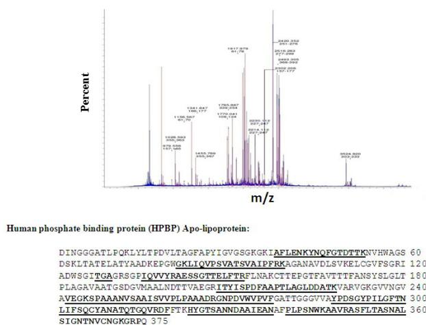
**Figure 6.** Mass spectrum of purified protein and peptides matched with human phosphate binding protein.
