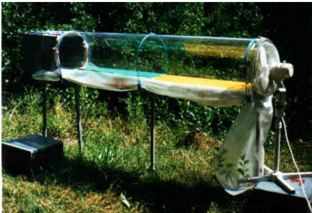
Figure 1. Wind tunnel made of transparent plexiglass, 2.20 m long with 0.42 m in inner diameter, with a fan at one end.
