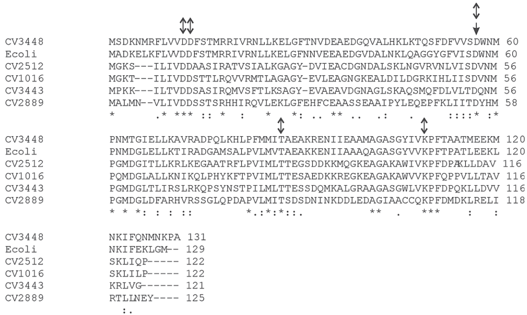
Figure 3. Alignment of the Chromobacterium violaceum deduced CheY and the homologue in E. coli . Single arrow indicates the phosphorylation site; double arrows indicate the conserved residues of the response regulator.
